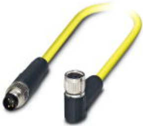
Sensor/Actuator cable, 4-position, PVC, yellow, shielded, Plug straight M8, on Socket angled M8, Cable length: 0.5 m
